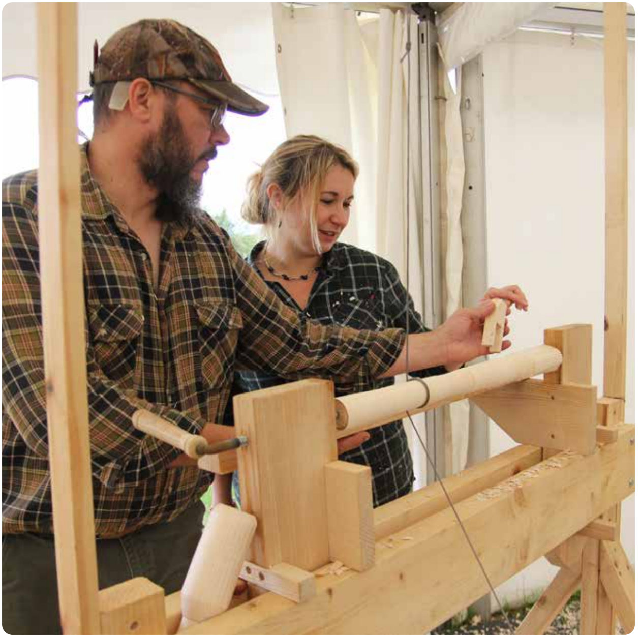
Shaping a stool leg on the pole lathe
